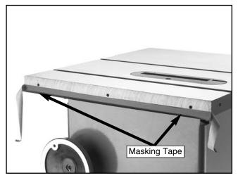
**Figure 9.** Using tape to shim for wing alignment.
